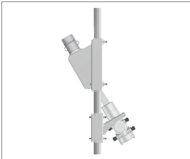
Fig. 16: 30° measurement setup on a pipeline with diameter 50 ... 100 mm (1.97 ... 3.94 in)
