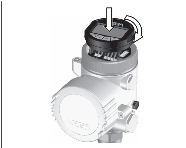
Fig. 21: Installation of the indicating and adjustment module
