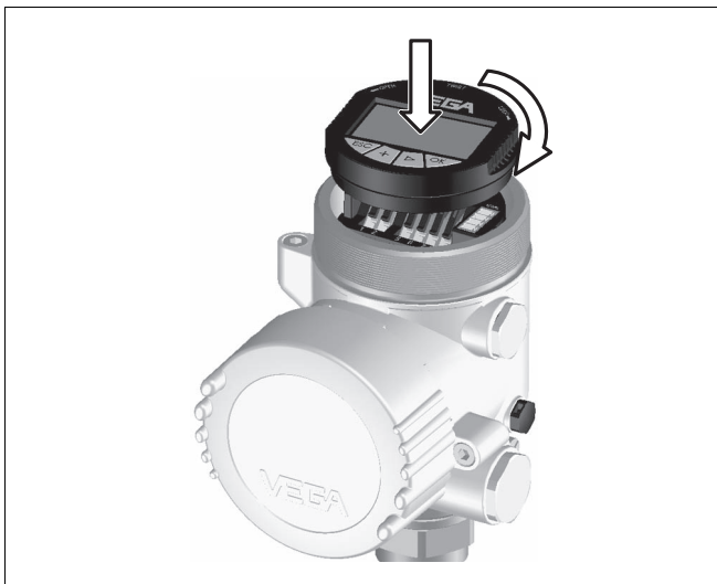
Fig. 21: Installation of the indicating and adjustment module
