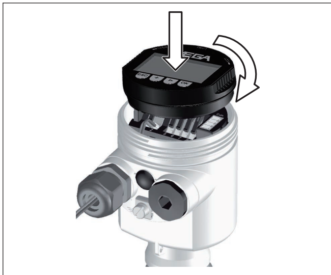
Fig. 25: Insert display and adjustment module in the single chamber housing
