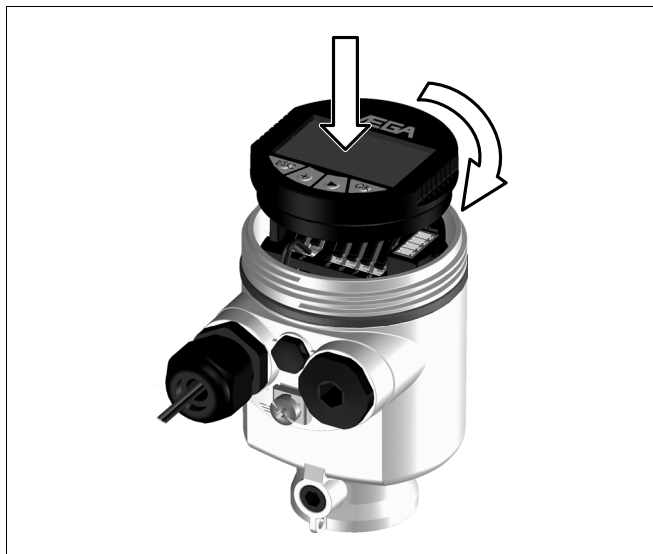
Fig. 14: Insert indicating and adjustment module
