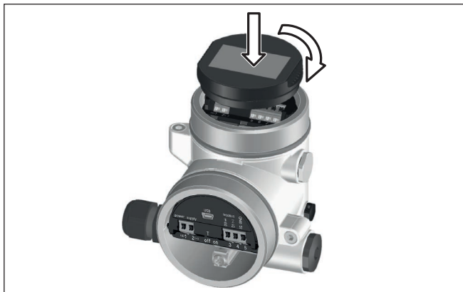
Fig. 15: Insertion of the display and adjustment module
