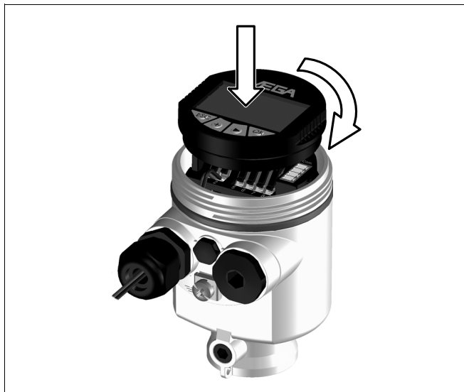
Fig. 24: Mounting the indicating and adjustment module
