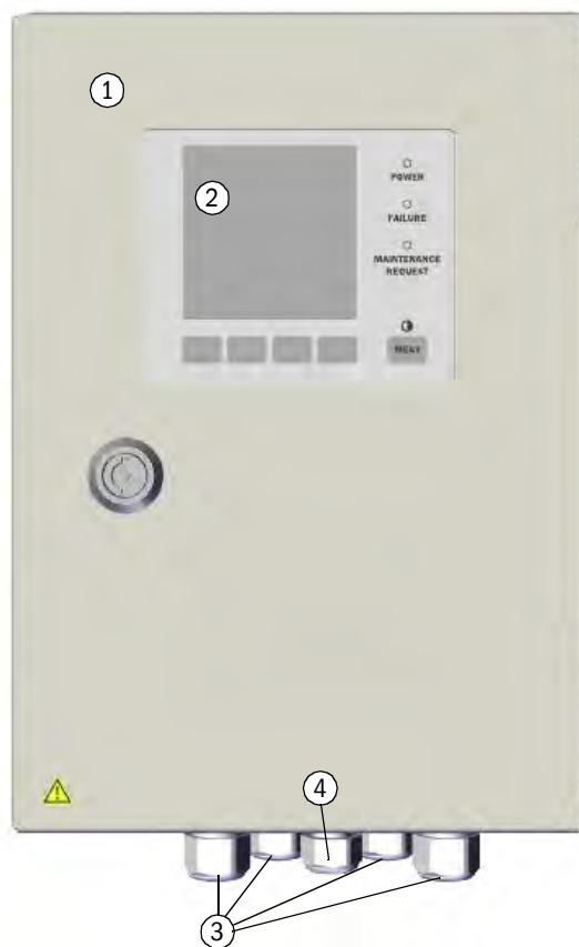
Fig. 6: TAD control unit
