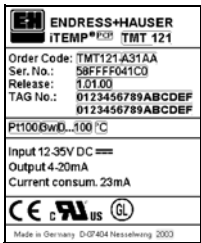
Fig. 1: Example: DIN rail transmitter legend plate
