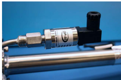
Figure B-10 Newly installed pressure sensor positioning
