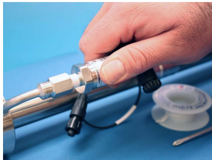
Figure B-9 Replacing pressure sensor
