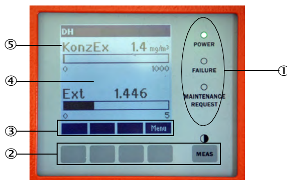
Fig. 50: Functional elements LC display of MCU control unit
