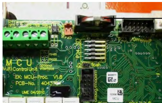
Fig. 53: Button cell exchange, MCU
