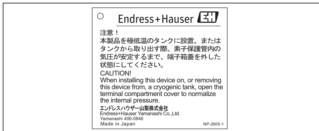
Figure 24: -170°C caution plate
