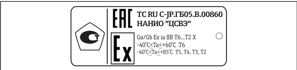
Figure 12: EAC approval nameplate
