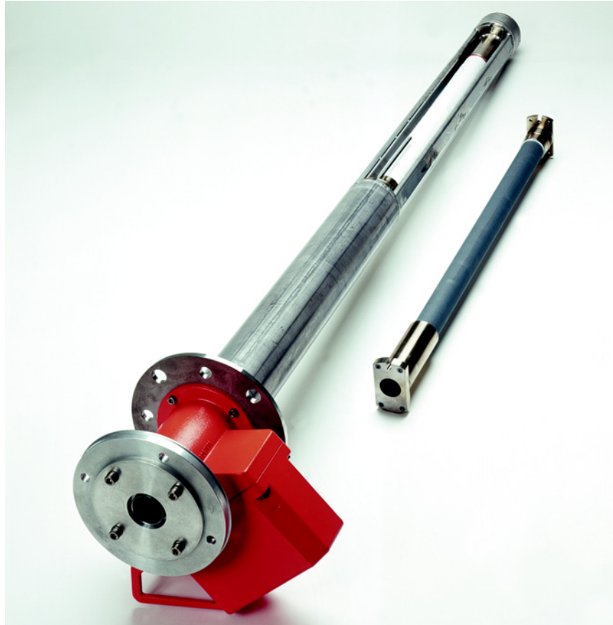
Fig. 3 GPP measuring probe with ceramic filter and ceramic/teflon filter
