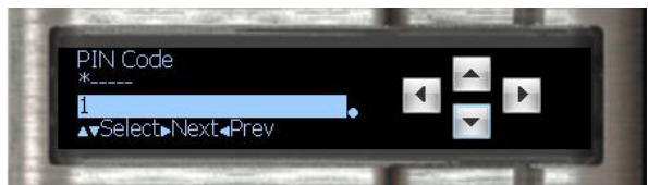
Fig. 23: Menu “Login” Flow-X module LCD display
