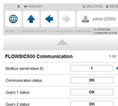
Fig. 29: Menu item "Communication/Flowsic600-XT Flow Meter/FLOWSIC600-XT Communication"
