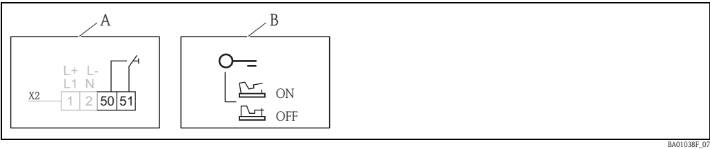
A Key to acknowledge demand mode in the interlocked state B Configuration via the interlock switch (ON/OFF)
