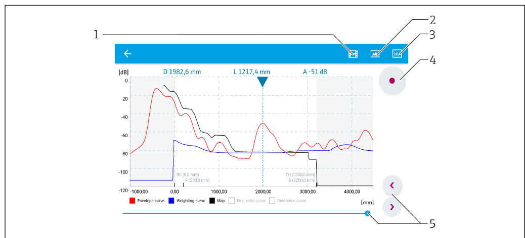
36 Envelope curve display (example) in SmartBlue; Android view
