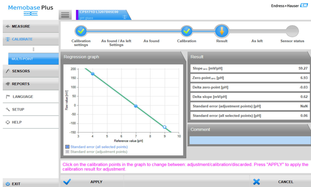
16 Multipoint calibration: buffers 4 and 7 selected as the adjustment points, buffer 9 as the calibration point
