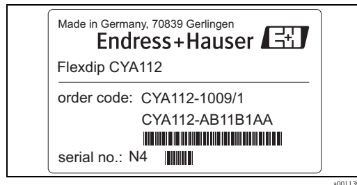
Fig. 1: Example of a nameplate
